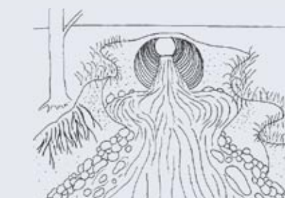
SCOURING AND EROSION Causes: Undersized or perched crossings
