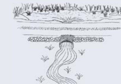
PONDING Causes: Undersized or perched crossings
